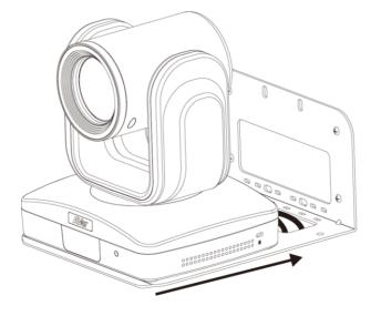
6. Screw tight the screw to secure the camera on the wall mount.
