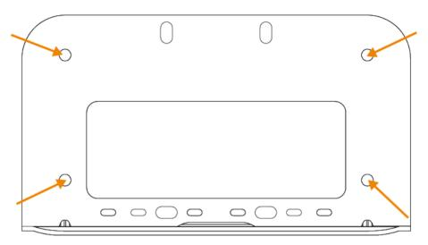
2. Secure the wall mount bracket on the wall within screws.
