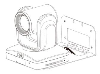
5. After connecting all cables, slide the camera in the end.
