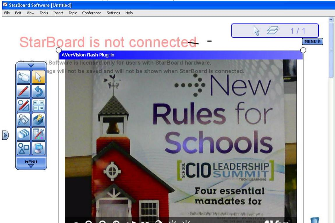
11. The controls in the lower portion (you must mouse over the portion for them to appear) of the application are for the following (where supported by your AVer document camera): Auto focus, zoom in/out, rotate, pause, mirror, brightness higher/lower.
