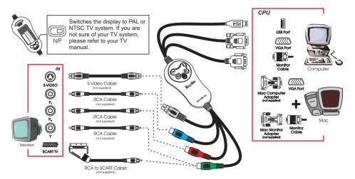
**WARNING**: Do not connect the S-video and the YP<sub>b</sub>P<sub>r</sub> at the same time. To avoid damaging the unit, operate this unit within a temperature range of 0° to 40°c (32°~104°f).
