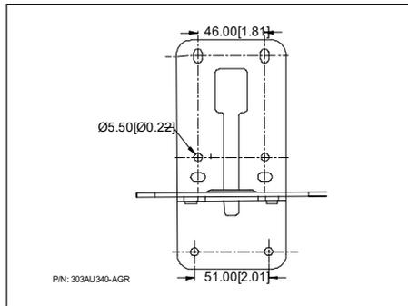
2. Use the screws (not included) to secure the L-mount bracket **A** on the wall.
