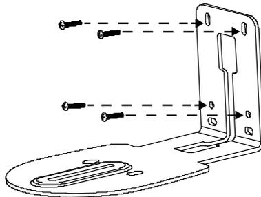
3. Then, assemble the L-mount brackets **A** + **B** with screws (included in package).
