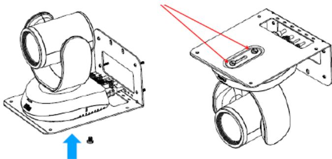
5. Find suitable screws to fix the camera mount to the ceiling.
