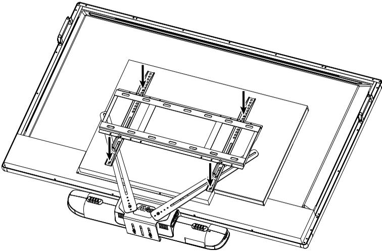
6. If users don't need to install mount rack of TV, then, secure the fixture on the TV. Then, adjust the fixture to an appropriate position if needed. Finally, tightly screw all screws.
