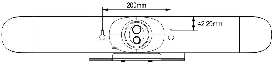
2. Use the supplied 2 Tripod Screws to secure the supplied Wall Mount Kit to the bottom panel of the camera.
