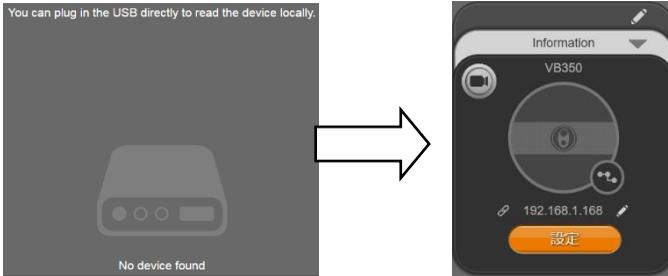
5. Set up IP address. The camera default IP address is 192.168.1.168. Click the pencil icon (✎) to edit IP address.
