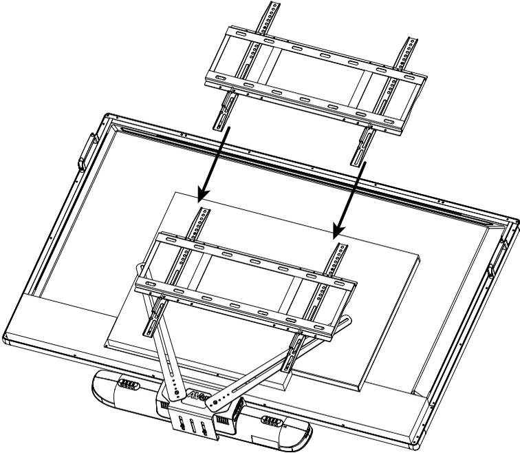
5. Secure the mount rack and fixture on the TV. Please do not screw tight at this stage. Then, adjust the mount rack and fixture to an appropriate position if needed. Finally, tightly screw all screws.
