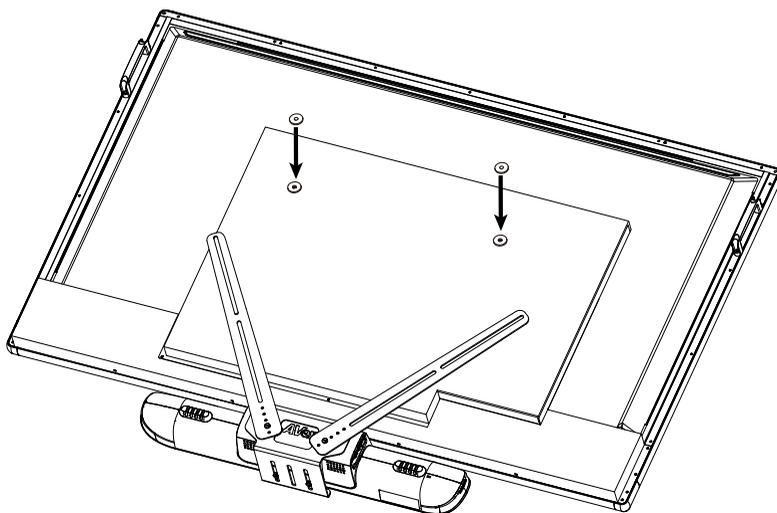
4. Place mount rack of TV on top of fixture.
