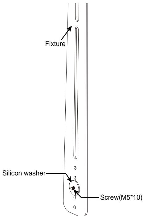
2. Secure the fixture on the rear side panel of the camera. Don't screw tight at this stage. You can select among the four screw holes for screwing the fixtures.
