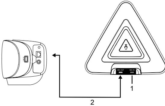
1. The port won't be used while using with VB350. It doesn't support daisy chain connection.
