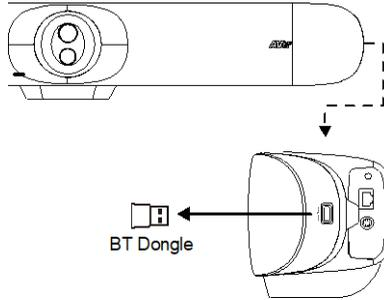
Install a BT dongle before powering up the device. Plug it into the USB 2.0 type-A port. Use remote control or PTZApp 2 to enable Bluetooth function.
