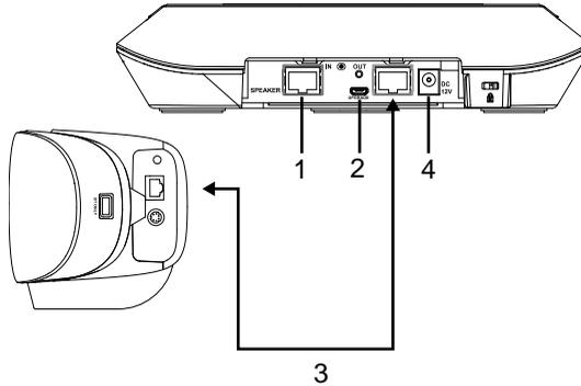
1. The port won't be used while using with VB350. It doesn't support daisy chain connection.
