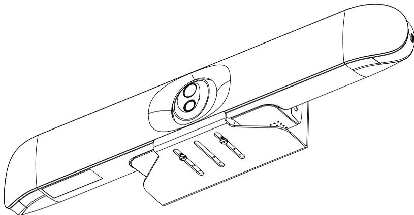
3. Align the mounting holes on the Wall Mount Kit with the two screws on the wall and hang the camera on the wall.
