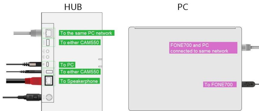
7. To activate the FONE700 Audio Tracing (Voice Tracking) feature, first connect the **CAM550** and set up the **Preset Link function with the FONE700**. After this setup, the Audio Tracking option will become available on the FONE700.
