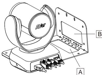
4. Turn the camera to face the front side. Install the second screw and tighten both screws.
