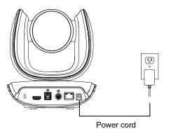
Connect the included power adapter and power cord to a wall outlet.
