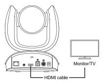
Connect with TV or monitor through the HDMI port to display camera video on the screen.
