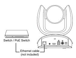
Or connect a CAT 5e FTP cable (not included) to the PoE Switch or Ethernet.
