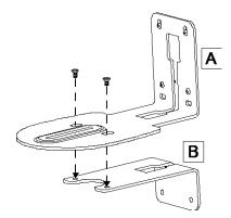
After assembling the L-mount brackets, use the screws (not included) to secure the lower part of L-mount brackets on the wall.
