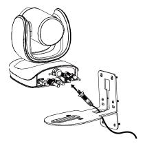
6. Use the remaining screws (included in package) to secure the camera on the L-mount bracket.
