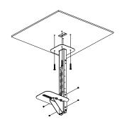
Connect all cables on the camera and pass all cables out through the hole on the mount bracket. Then, secure the camera on the camera bracket.
