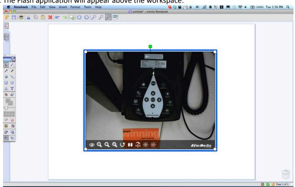
11. The controls in the lower portion (you must mouse over the portion for them to appear) of the application are for the following (where supported by your AVer document camera): Auto focus, zoom in/out, rotate, pause, mirror, brightness higher/lower.
