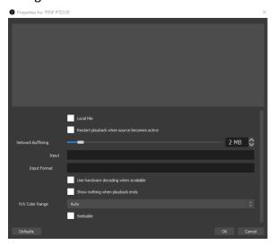
10. Next, in the "Input" field, type in the following syntax for the TR310/333 RTSP feed, "rtsp://Camera IP:554/live\_st1", where Camera IP is the actual IP address of the camera.
