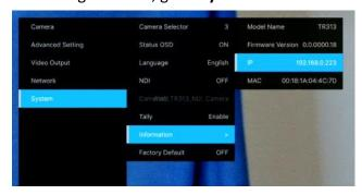
2. Once you have the IP address setup, type the IP address in your Chrome browser (Setup on same subnet) and you should now see the login to the TR310/333 camera shown below.
