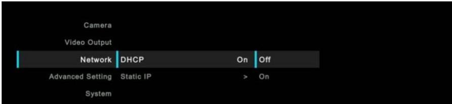
After turning DHCP on, go to **Information** to view the IP address.
