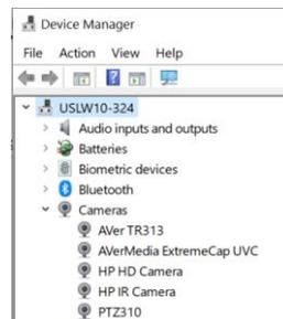
**USB Connection (TR313V2):** Connect the AVer TR313V2 Camera to a USB port on the PC using a Type-B USB cable to Type-A/C USB cable and verify that Windows does see the device in the “Device Manager” window.
