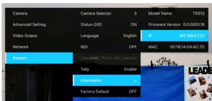
2. Once you have the IP address setup, type the IP address in your Chrome browser (Setup on same subnet) and you should now see the login to the TR313 camera shown below.
