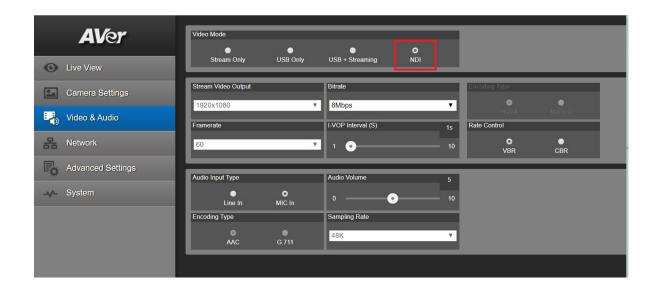
\*Note: The STREAM Video Output, Framerate, Encoding type, and Sampling Rate settings are only for viewing, they are not adjustable in NDI mode. The NDI native video resolution is 1920x1080P /60.
