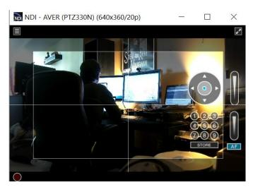
4. The NDI AVer camera controls are Pan, Tilt, Zoom, Manual Focus, Automatic Focus, and Position Presets.
