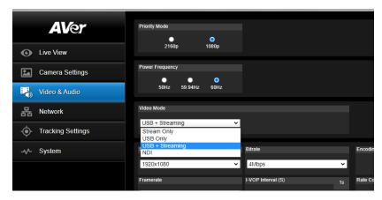
\*Note: The STREAM Video Output, Framerate, Encoding type, and Sampling Rate settings are only for viewing, they are not adjustable in NDI mode. The NDI native video resolution is 1920x1080P /60, but is adjustable in the TR camera, 30fps / 60fps etc. The TR Camera will have an SDI/HDMI output in ALL modes.
