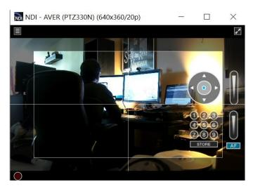
4. The NDI AVer camera controls are Pan, Tilt, Zoom, Manual Focus, Automatic Focus, and Position Presets.
