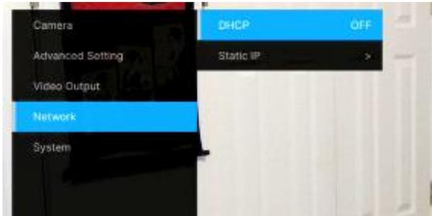
After turning DHCP on, go to **System > Information** to view the IP address.
