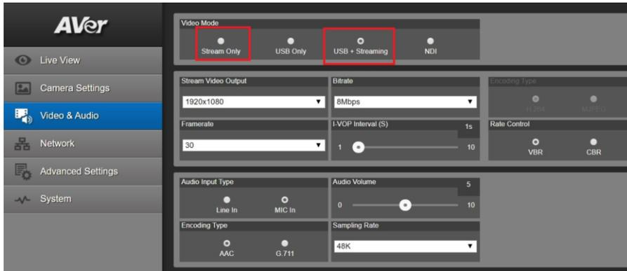
**\*Note:** Once streaming has started do not change the Stream Video Output on the fly, you will need to “Stop” streaming, change the Stream Video Output, then “Start” the stream again.
