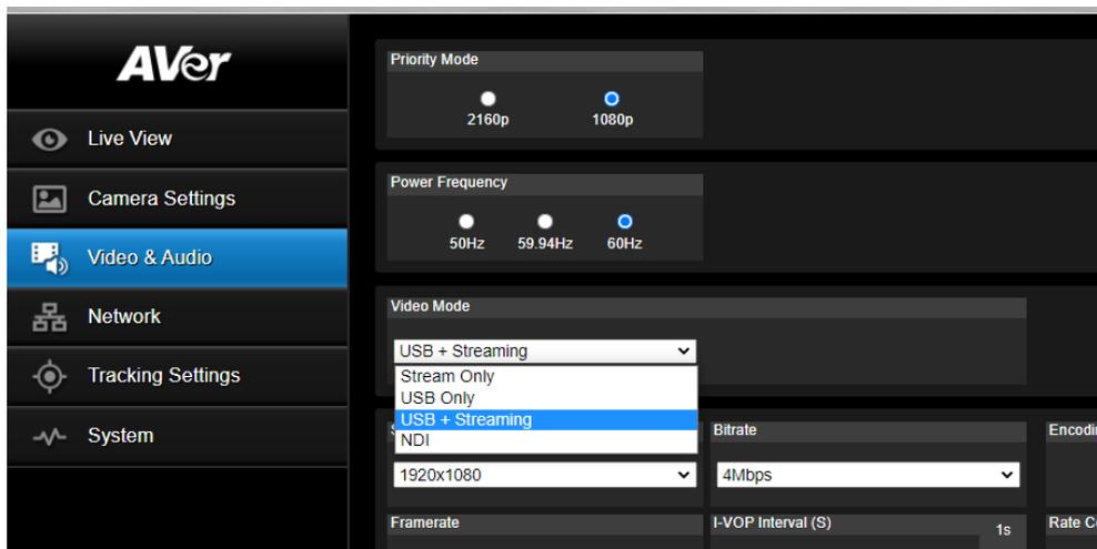
**\*Note:** Once streaming has started do not change the Stream Video Output on the fly, you will need to “Stop” streaming, change the Stream Video Output, then “Start” the stream again.
