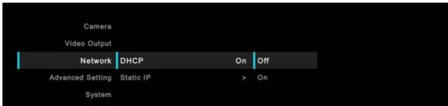
After turning DHCP on, go to **System > Information** to view the IP address.
