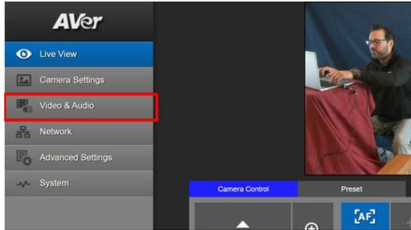
5. Next, after selecting the *Video & Audio* setting, verify that you have either “Stream Only” selected or “USB + Streaming” selected. Select your Stream Video Output standard, Bitrate, Framerate, Encoding, etc. **\*Note:** Some servers require minimum bitrate of 2.5Mbps for their environment.
