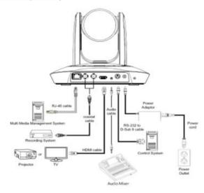
1. Connect the TR530 camera via RJ45 Network Cat5E (or better) cable; verify IP address of Camera in order to connect via Web browser. If IP address is not known, locate the remote, select the "Menu" icon and navigate to the "Camera->DHCP->" setting, verify DHCP is set to "On" in order to grab an available IP address. If you are reserving IP addresses, verify it is set to "OFF" and that the correct IP address has been set.
